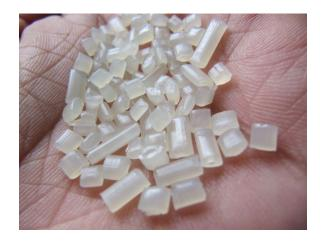
Compared to Polyethylene Terephthalate, Polypropylene (PP) has a lower degree of clarity. Like PET, PP is a durable and tough material, and is resistant to heat, chemicals, and oil. In applying to the beverage packaging, PP cup (also known as translucent cup) is semi-transparent in color.
