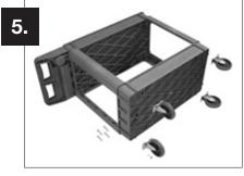
Use 4 bolts, lock washers and nuts to secure legs and casters to frame
