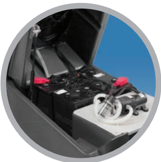
Gel batteries are standard
