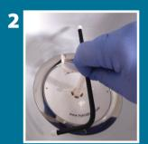
Twist removal tool clockwise onto center stem of the cartridge until snug. Do not over-tighten.
