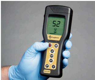
1. Turn On and Allow Meter to Calibrate
